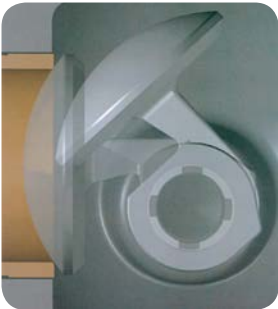
Conventional Valve Design 1:1 ratio of forces requires large actuator
