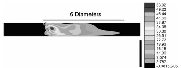
**Fig. (10b).** Turbulent kinetics energy downstream the mixer. Air system, pipe diameter 2".
