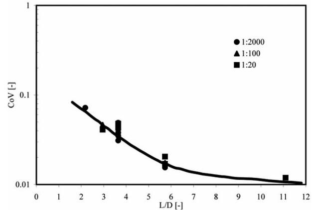
Fig. (7). Mixing in a pipe after the fluid outlet from the CompaX mixer. Air CO<sub>2</sub> system, pipe diameter 6” Laser, test method induced fluorescence (LIF).
