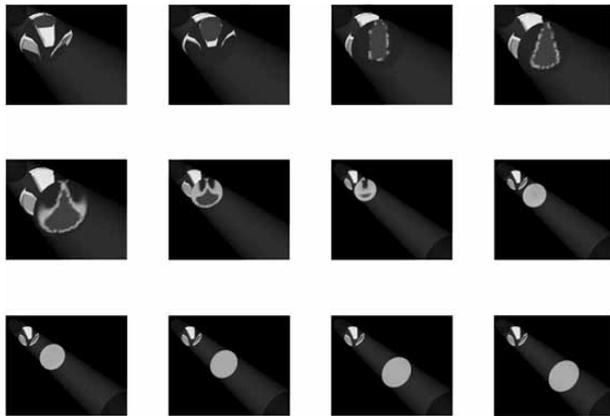
Fig. (6). Evolution of the additive dispersion along the pipeline .
