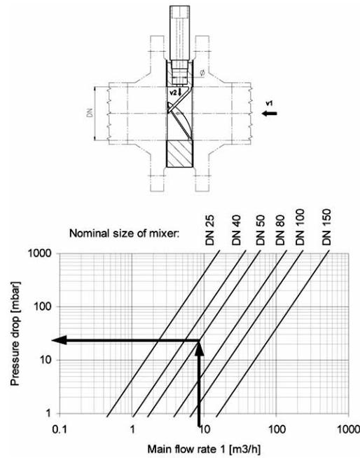
Fig. (11). Suggested guidelines for selecting the nominal diameter of the mixer.
