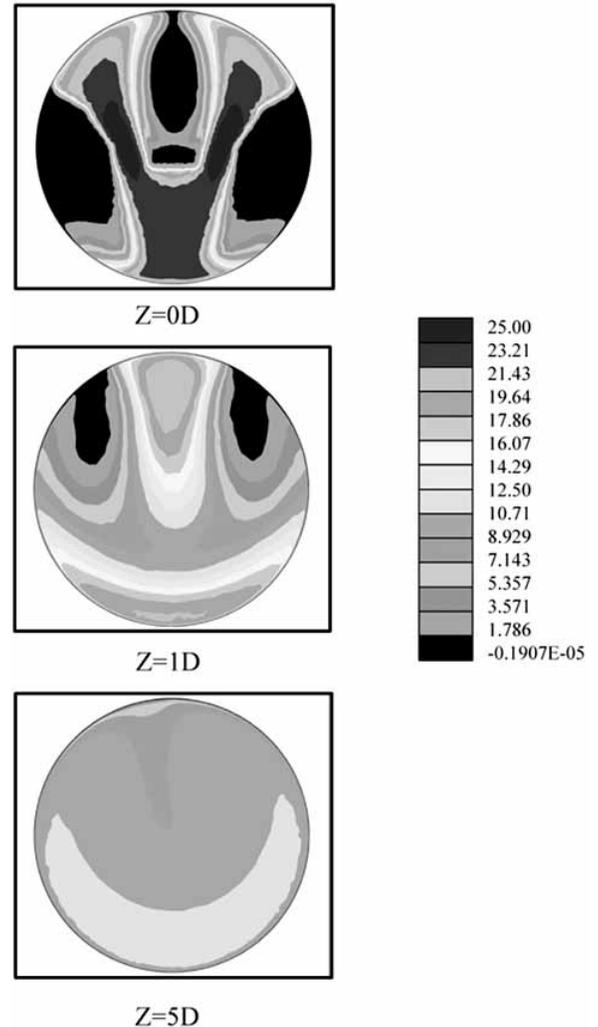
**Fig. (10a)** Velocity distributions at 0, 1 and 5 diameter downstream the mixer. Air system, pipe diameter 2".
