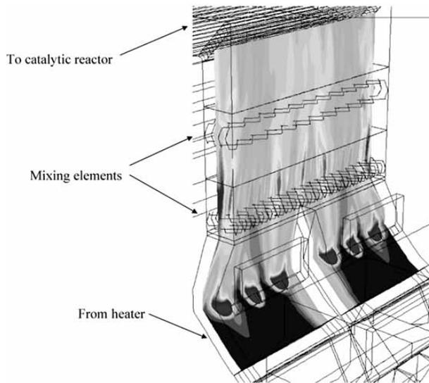
Fig. (2). Temperature homogenization upstream of a flue gas heater in a DeNOx process [8].
