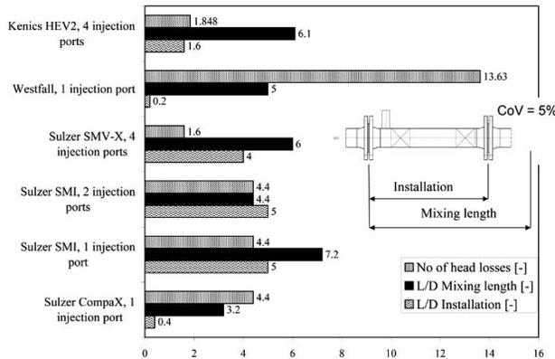
Fig. (14). Comparison of mixer efficiencies. Experimental conditions:  $CoV < 0.05$ ,  $V_1/V_2 \sim 1000$ ,  $Re > 10^4$ .
