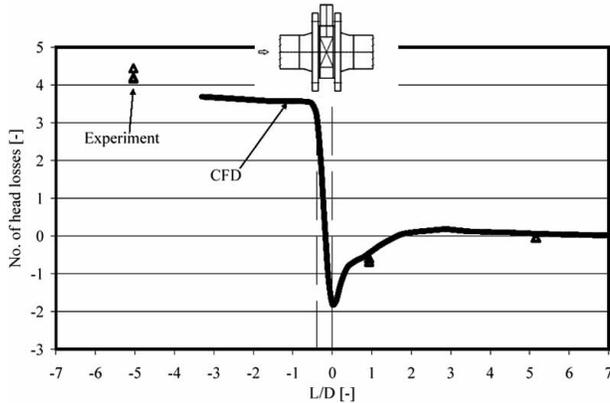
**Fig. (9).** Pressure drop across the CompaX mixer, experimental and computed trends. Air system, pipe diameter 2", standard k-ε model, incompressible flow, unstructured grid.
