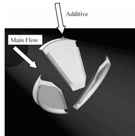
Fig. (4). A schematic diagram of the CompaX mixer.
