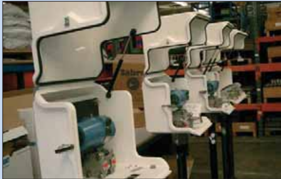
IEX1 Enclosures with integral manifolds and transmitters
